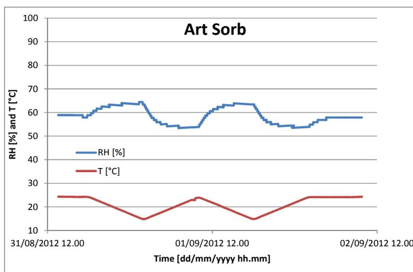
Figure 5: T and RH measured inside the case conditioned with Art Sorb®
