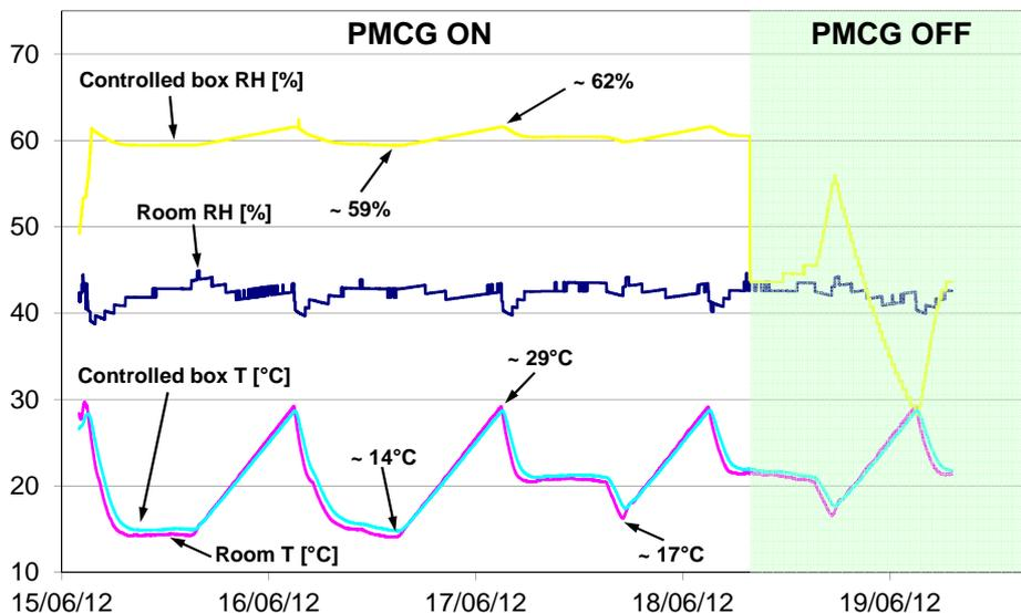
Figure 3: Test performed in fluctuating temperature conditions setting a mild target inside the case and a low relative humidity in the external environment.
