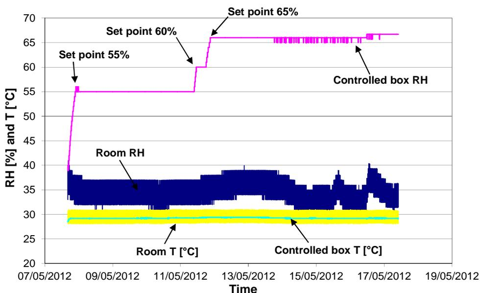
Figure 2: Test performed at constant environmental conditions with a high temperature setting a mild target inside the case and a low relative humidity in the external environment.
