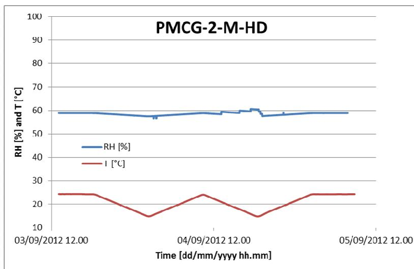
Figure 7: T and RH measured inside the box conditioned with PMCG unit
