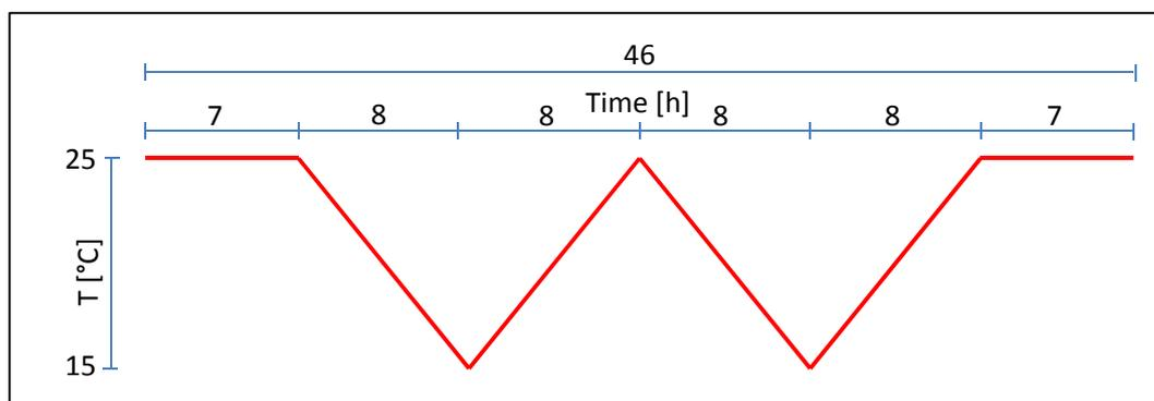
Figure 1: The temperature cycle and the scheduling of the tests
