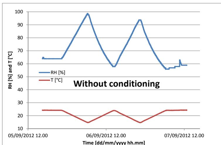
Figure 4: T and RH measured inside the case without conditioning
