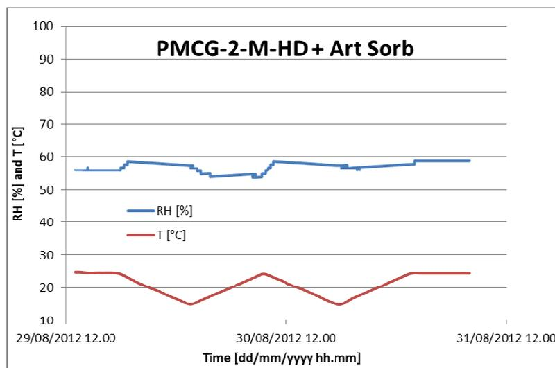
Figure 6: T and RH measured inside the case conditioned with PMCG unit and Art Sorb®
